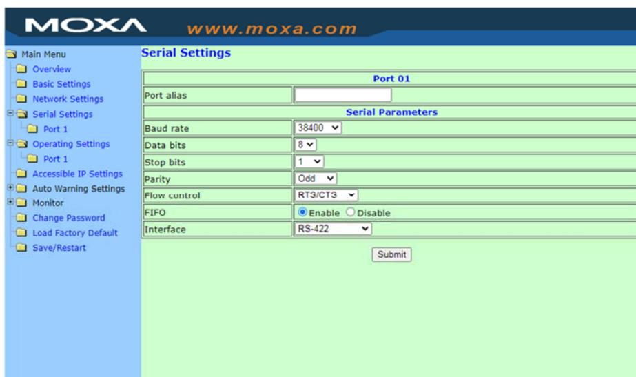
The screenshot shows the MOXA web interface for Serial Settings. The left sidebar is the same as in Figure 1. The main content area is titled 'Serial Settings' and shows 'Port 01' configuration. It includes a Port alias field and a 'Serial Parameters' section with dropdown menus for Baud rate (38400), Data bits (8), Stop bits (1), Parity (Odd), and Flow control (RTS/CTS). There are radio buttons for FIFO (Enable selected) and a dropdown for Interface (RS-422). A Submit button is at the bottom.
